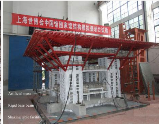
Model tests on shaking table
